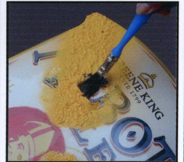
Application of Paint Stripper
